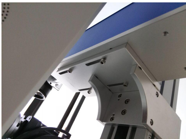
Computer installation on the machine cabinet
