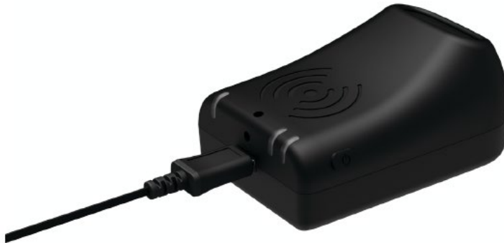
Picture 1 Charging Nordic ID EXA31 via USB charger
