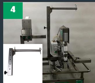
First slide the roll with the male tags over the support, please be aware of the rolling as shown on the picture below, counter clockwise:
