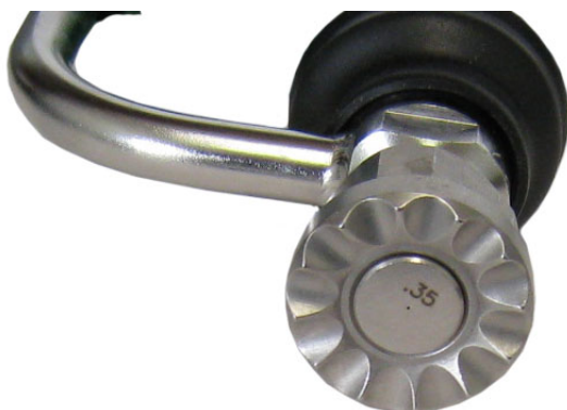
Nozzle in correct position
