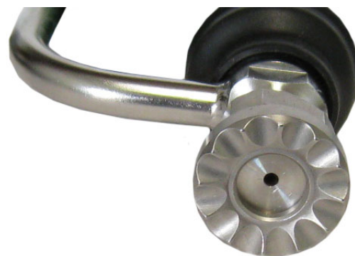
Nozzle back-to-front for cleaning
