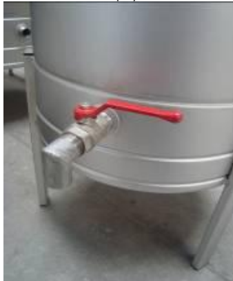
Photo. Run-out at the bottom of the tank.
