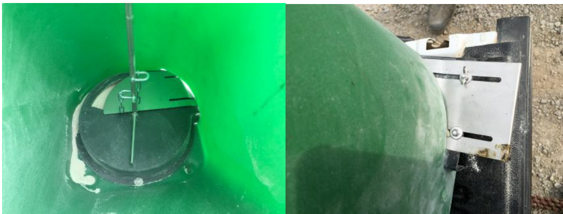
The dosing plate mounted on the MS Spreader
