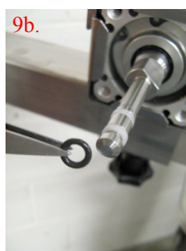
← (left) Remove the old (worn) o-ring. (right) → Fit the new o-ring over the piston, in front of the white ring.
