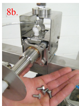
Remove the piston housing complete with reservoir from the Oral Dispenser.
