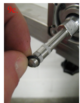
← (left) Remove the old (worn) o-ring. (right) → Fit the new o-ring over the piston, in front of the white ring.
