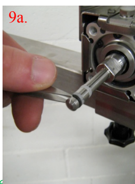
Unscrew the four piston housing bolts.
