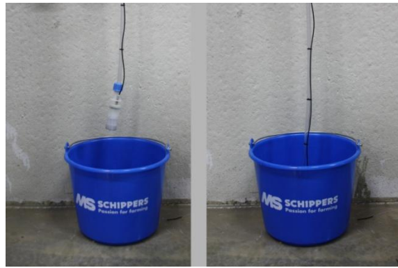
Figure 6: Put the suction hose in the liquid
