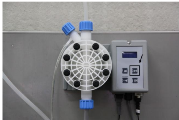
Figure 8: Filling the pressure hose
