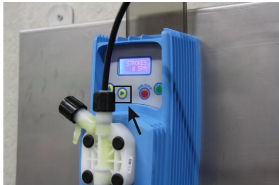
Figure 12: Filling the pressure hose
