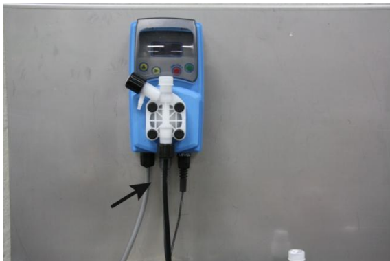
Figure 3: Connecting the suction hose
