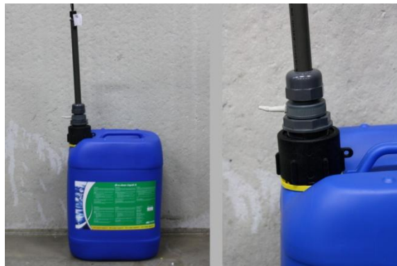
Figure 10: Connecting the suction lance to the
