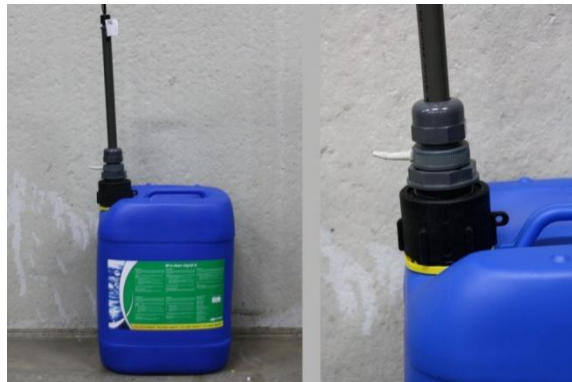
Figure 6: Connecting the suction lance to the
