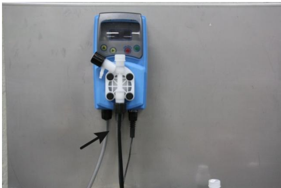
Figure 3: Connecting the suction hose
