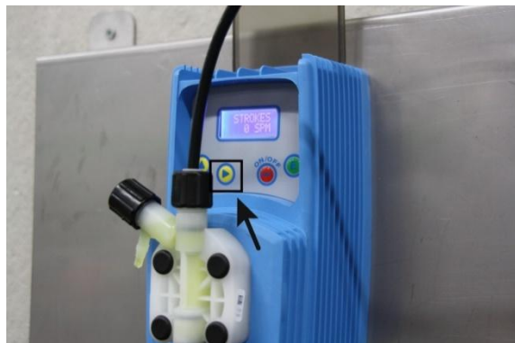
Figure 8: Filling the pressure hose
