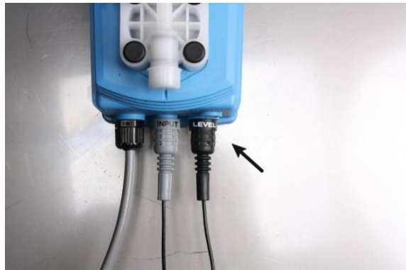
Figure 2: Connect the dry-run protection and
