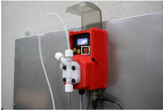
Figure 5: Switching the pump on
