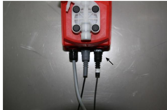
Figure 2: Connecting the dry-run protection
