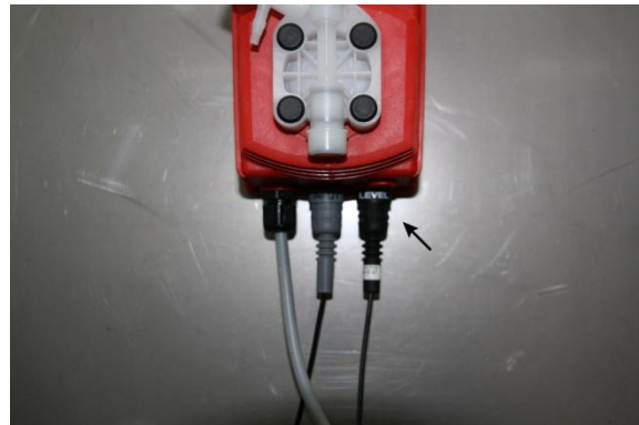
Figure 6: Connecting the dry-run protection
