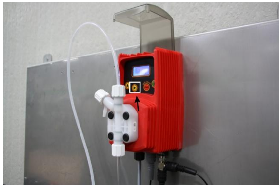
Figure 16: Filling the pressure hose
