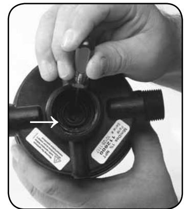
Step 6. Replace #17 O-ring.
