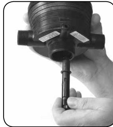
Step 5. Replace #17 O-ring.
