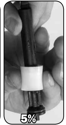
Step 3. Replace #44 DOSAGE PISTON thin lips up. Clean & inspect #14 O-ring replace if necessary.
