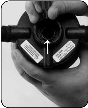
Step 4. Remove #17 O-ring and replace.
