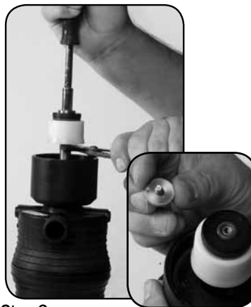
Step 2. Unscrew to unlock and remove #93 CAPSCREW.
