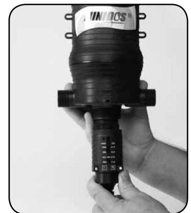
Step 9. Screw #7 OUTER CYLINDER onto body.
