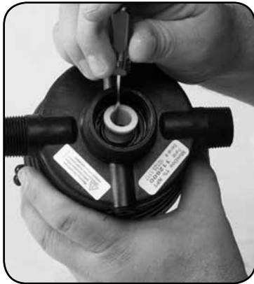
Paso 4. Remove #82 SHAFT SEAL SPACER.
