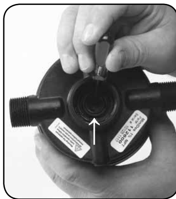
Step 5. Remove #17 O-ring and replace.
