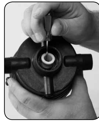
Step 3. Remove #83 SHAFT SEAL SPACER.
