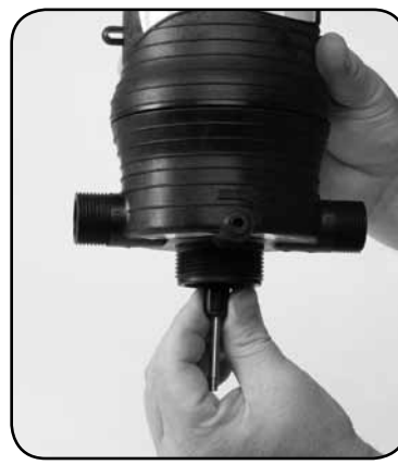
Schritt 8. Replace #51 SHAFT ASSEMBLY.
