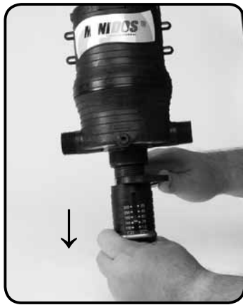
Paso 1. Unscrew #7 OUTER CYLINDER from body.
