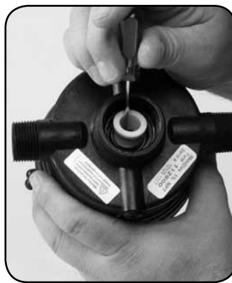
Step 5. Replace #83 SHAFT SEAL SPACER.
