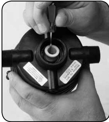
Schritt 4. Remove #82 SHAFT SEAL SPACER.
