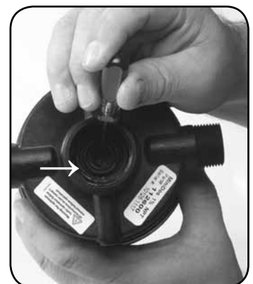
Schritt 6. Replace #17 O-ring.
