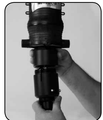
Step 9. Screw #61 OUTER CYLINDER onto body.
