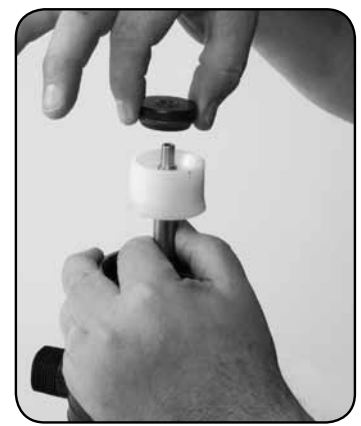
Step 3. Remove #73 DOSAGE PISTON GUIDE, clean and inspect #14 O-ring.
