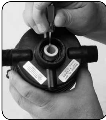
Step 4. Remove #82 SHAFT SEAL SPACER.
