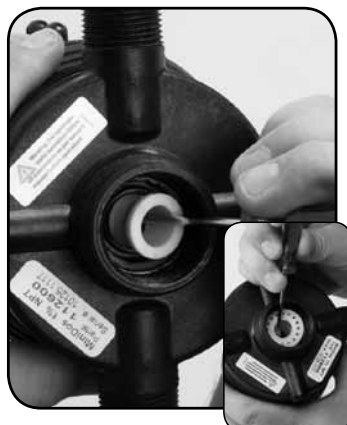
Paso 7. Replace #82 SHAFT SEAL SPACER and #16 Gasket.
