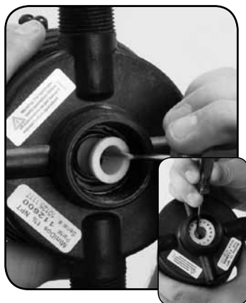
Step 7. Replace #82 SHAFT SEAL SPACER and #16 Gasket.
