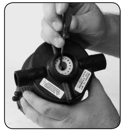
Step 3. Remove #16 Gasket.
