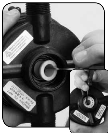
Schritt 7. Replace #82 SHAFT SEAL SPACER and #16 Gasket.
