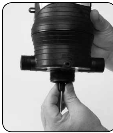
Paso 8. Replace #51 SHAFT ASSEMBLY.
