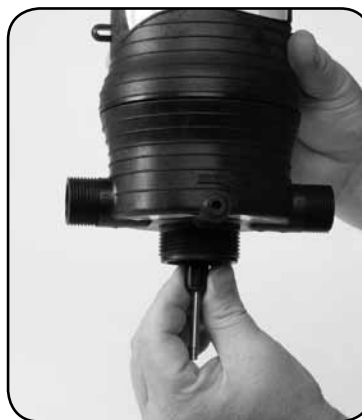
Step 8. Replace #51 SHAFT ASSEMBLY.
