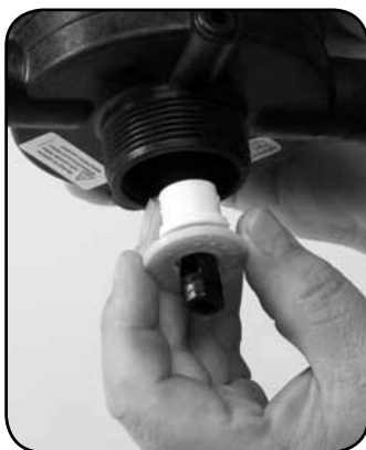
Step 7. Re-install #82 SEAL SPACER and #16 GASKET.
