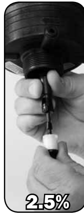
Step 2. Rotate #51 or #52 SHAFT 90° and remove.
